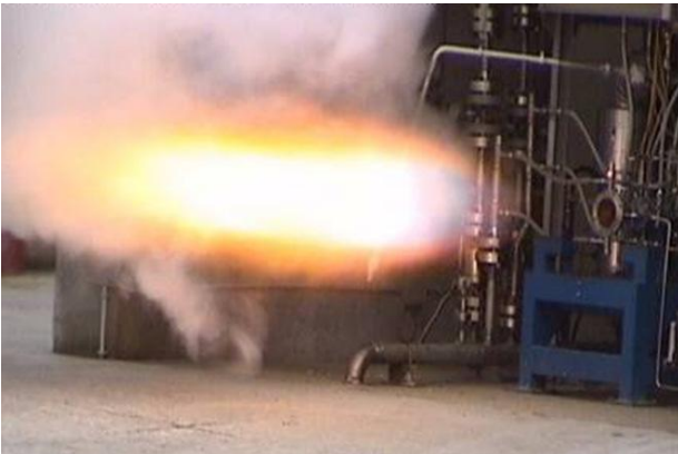
Fig.7 – Mira engine – sub-scale development test
