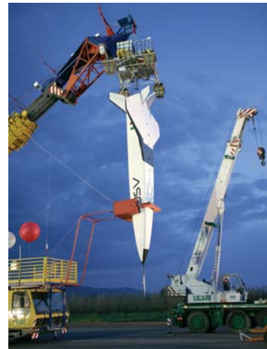
Figure 2. FTB_1 and gondola suspended from the launch machine before flight.
